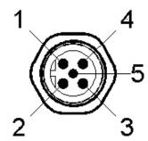
Please note that to replace ND valves with a ED version on a the standalone version the two 0V connections of the ND type must be bridged as the ND version uses only a common 0V.
