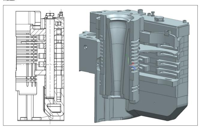
With the TRC system, the cooling nozzles are at equal distance to the outer mold diameter for both DG cavities. The nozzles are also "travelling" together with the Blank molds during the open/close motions, so that an equal distance between the cooling nozzles and the molds is kept during the full 360° cycle: in comparison with the old
