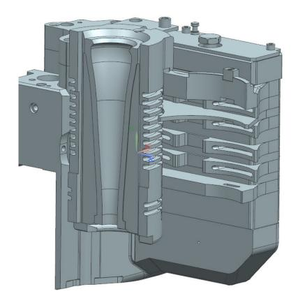
Mold transition IS 5 ½ " DG to AIS 6 ¼" DG – Travelling Radial Cooling
