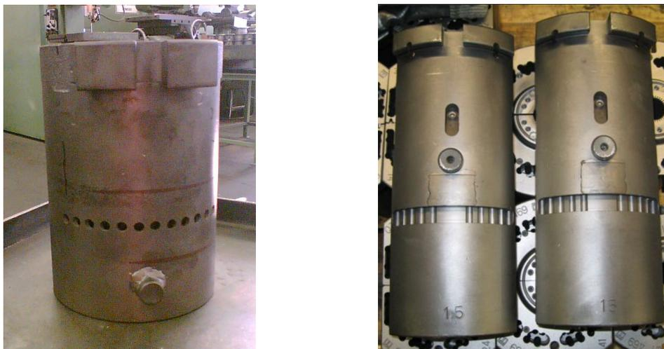
**Figure 3 - Implementation of supply bores in the mold using bores (left – example for an IS type machine) and a cut out (right - example for an NIS type machine)**
