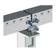
Beams above 5.5 meters are supplied in two pieces with jointing plate, adjusting brackets and an additional center support.
