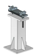
The Support provides adjustment for height, Leveling and positioning to the lehr input roller as shown.
