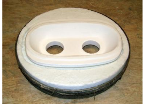
A complete orifice ring assembly with pan, pre-formed insulation, and orifice ring.
